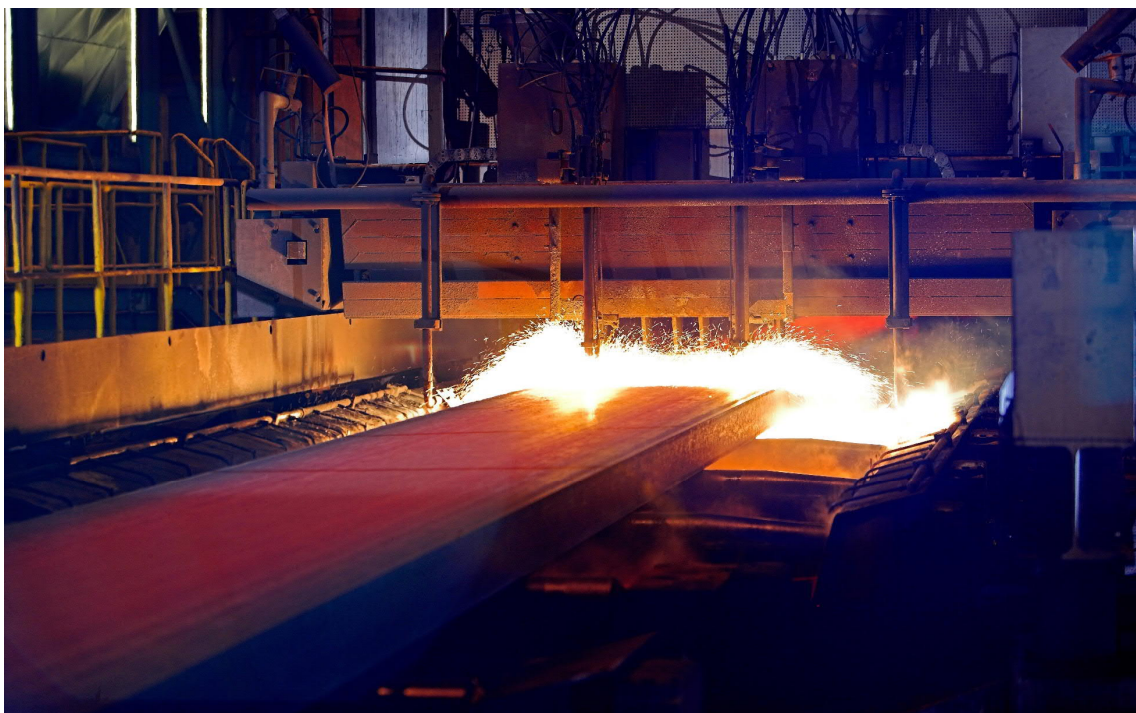
Torch cutting at a Primetals Technologies stainless steel caster
