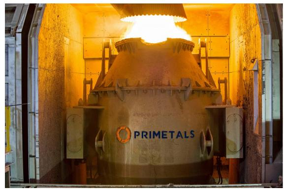
New argon oxygen decarburization (AOD) converter supplied by Primetals Technologies at the German steel producer BGH Edelstahlwerke GmbH in Freital, Saxony, Germany.
