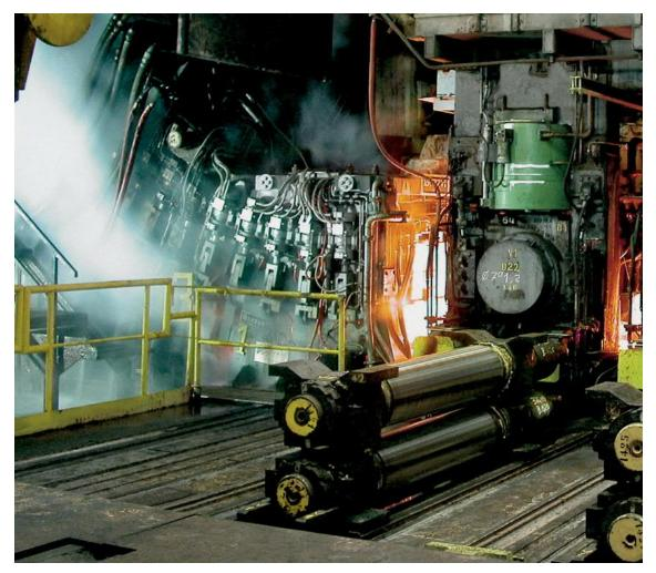
LevCon Bender Anti-Bulging by Primetals Technologies: A new process stabilizes the mould level by controlled oscillations of the bending zone.
