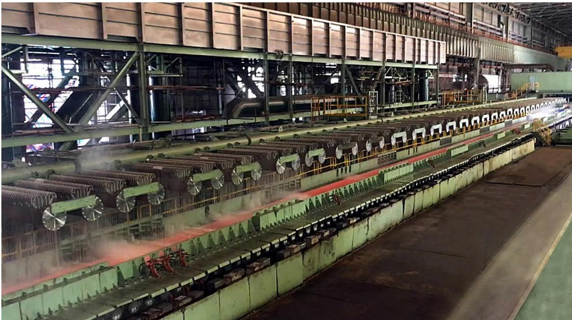
New laminar strip cooling implemented by Primetals Technologies at Baosteel
