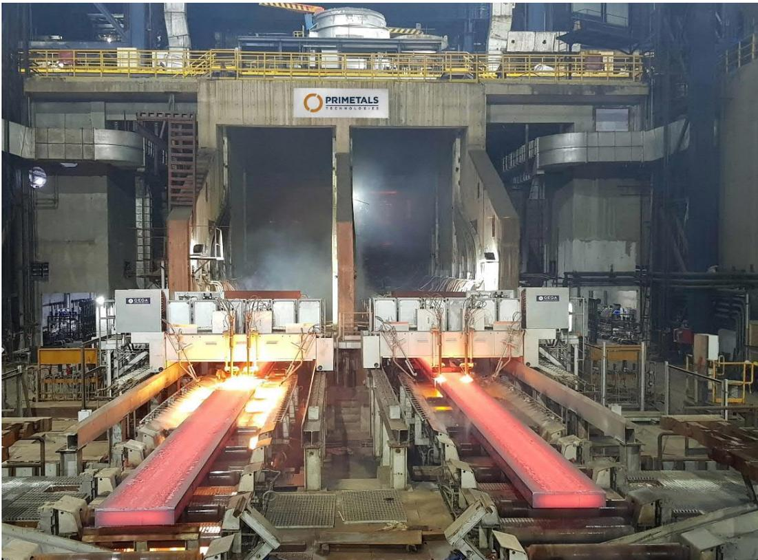
Continuous slab caster from Primetals Technologies installed in the Dolvi plant of JSW Steel in India.
