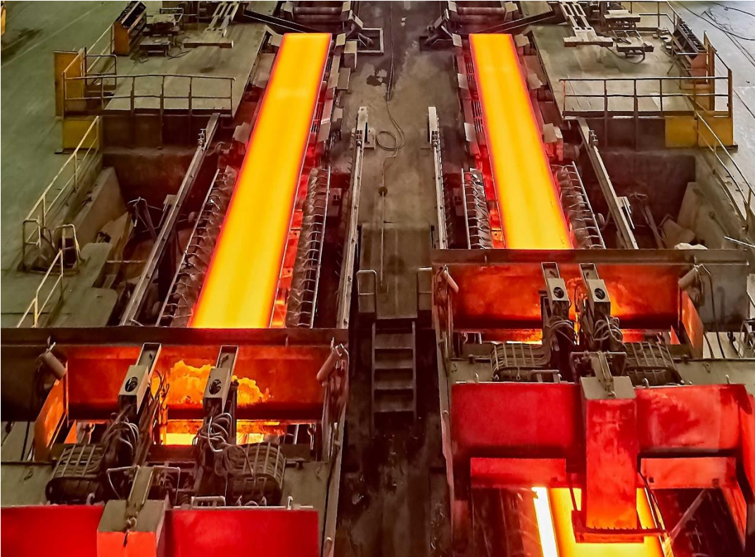
Çolakoğlu's 2-strand slab caster at its world record-setting plant in Dilovası, Turkey.
