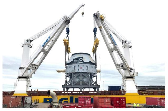
The 330-ton LD converter (BOF) from Primetals Technologies is lifted onto the cargo ship Happy River in the Rotterdam harbour.
