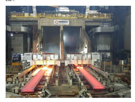
JSW Steel's two new slab casters from Primetals Technologies at the Dolvi steel plant.
