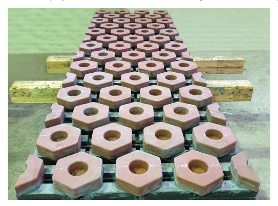
Copper staves with hexagonal inserts from Primetals Technologies ready for inspection prior to delivery.
