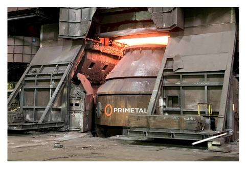
The new 125-ton LD converter (BOF) at ArcelorMittal Zenica's steel plant ensures increased productivity and has eliminated a sloping issue.
