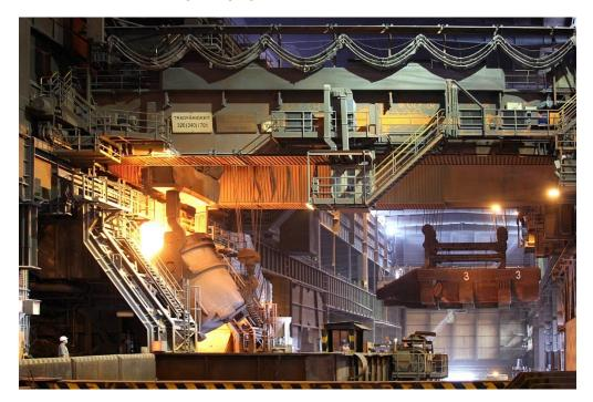
Converter charging at Salzgitter Flachstahl. Primetals Technologies has recently implemented the Slag Expert module at two LD converters (BOFs) in Salzgitter, Germany.
