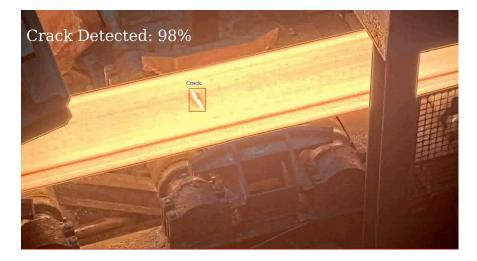
The digital assistant uses AI to detect strip cross cracks and instantly alerts operators to such defects.
