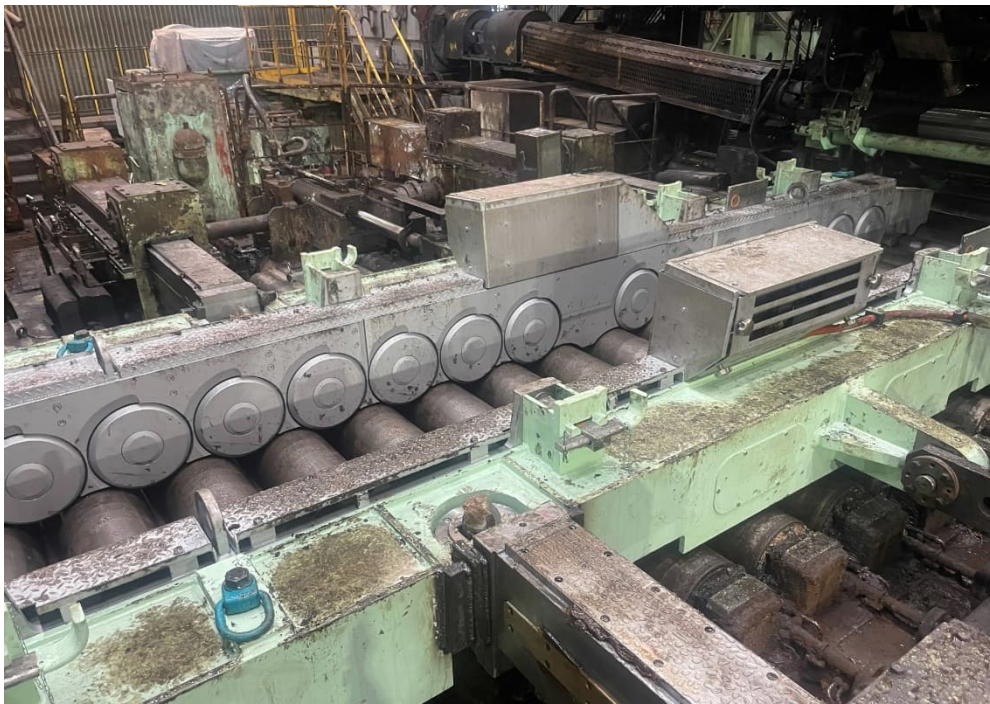
The newly implemented Eco Slides Discs and one of the new guiding beams.
