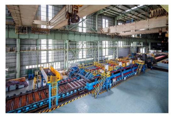
MULPIC, a world-leading plate cooling technology from Primetals Technologies.
