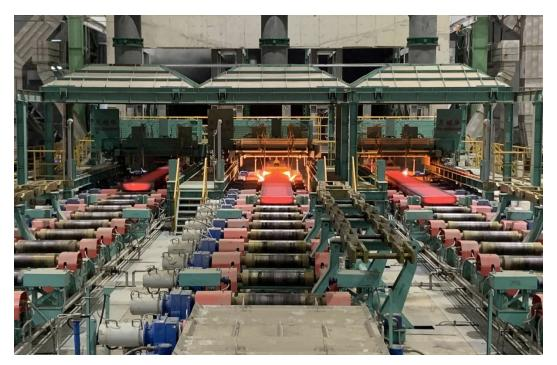
The world's first 3-strand continuous slab caster, supplied by Primetals Technologies, in operation at Chinese steel producer Tangshan Donghua.
