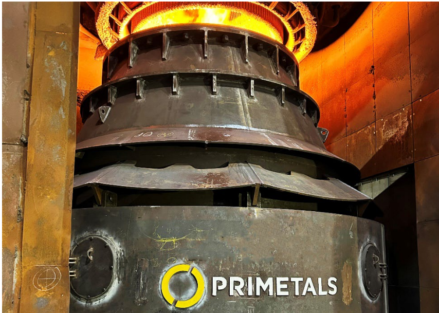
Primetals Technologies' revamped LD converter (BOF) No. 4 at voestalpine's Donawitz plant during the first heat.
