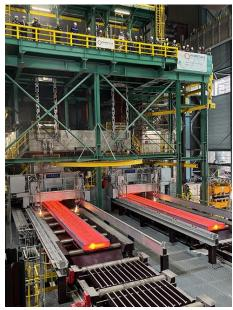
thyssenkrupp Steel's new continuous caster No. 4 from Primetals Technologies features advanced mechanical and automation solutions.
