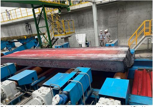
Primetals Technologies' new continuous caster at Wuyang Iron and Steel is engineered to produce ultra-thick slabs up to 460 millimeters thick.
