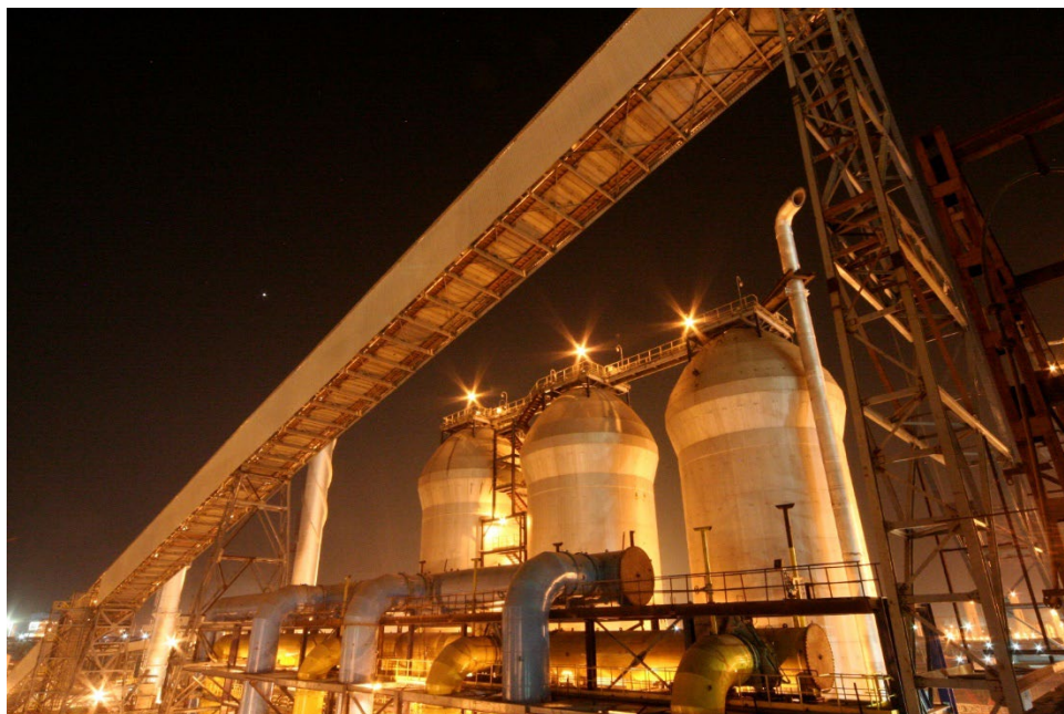
Internal-combustion stoves from Primetals Technologies installed in India.
