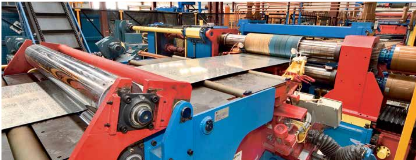
Slitting line at BlueScope Steel, Perth, Australia
