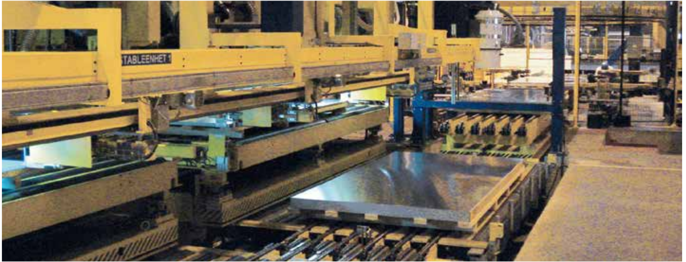
Cut-to-length line, Hydro Aluminium, Norway
